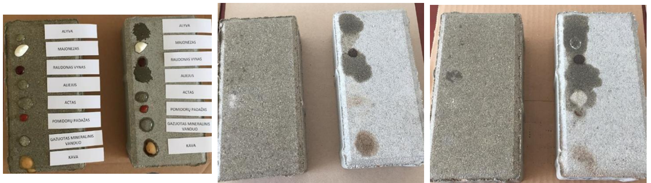
This photo shows the liquids used for the stain test.
