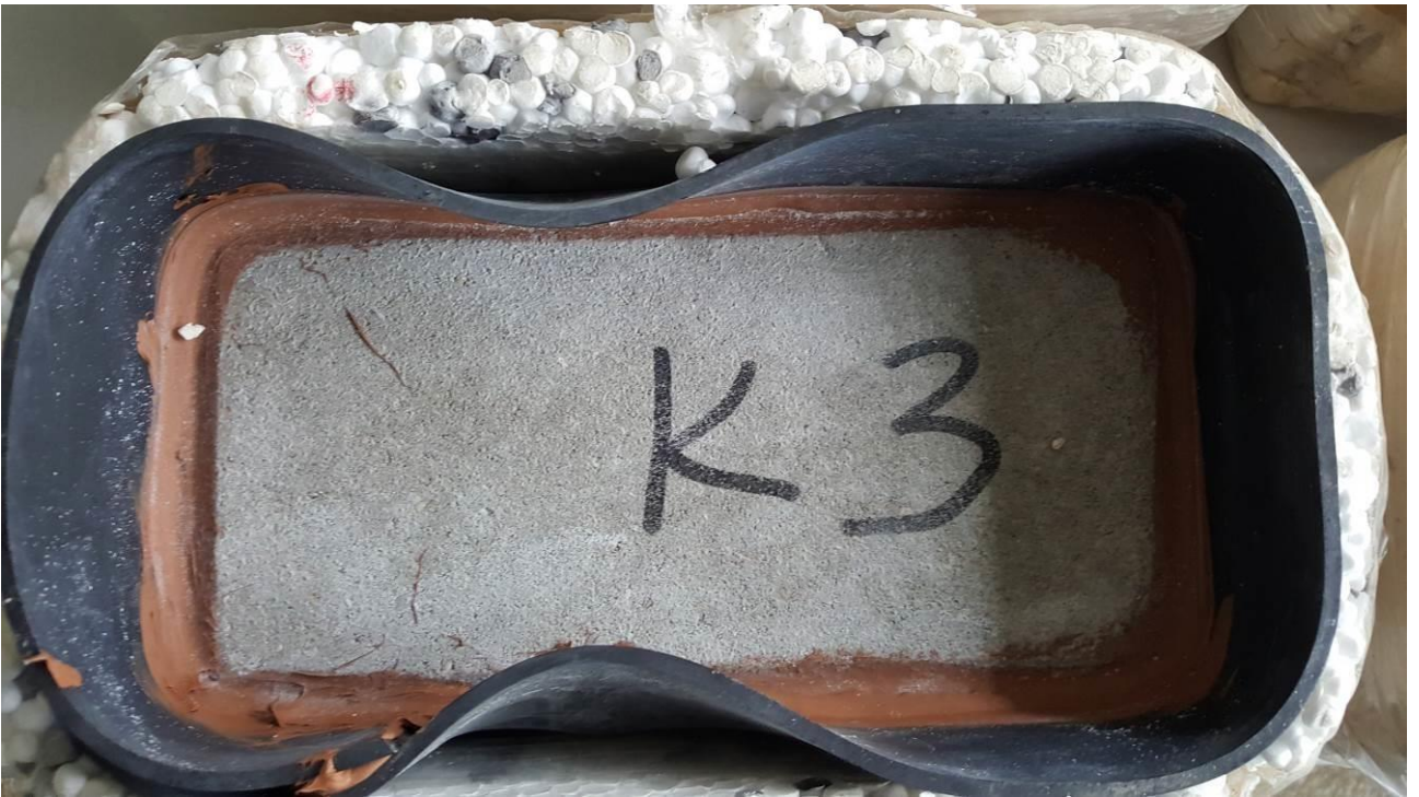
9 Figure Block K3 before the freeze/thaw testing (top) and after 72 days of testing (bottom)
