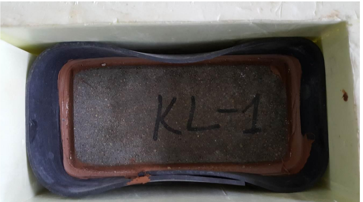
3 Figure Block KL-1 before the freeze/thaw testing (top) and after 72 days of testing (bottom)
