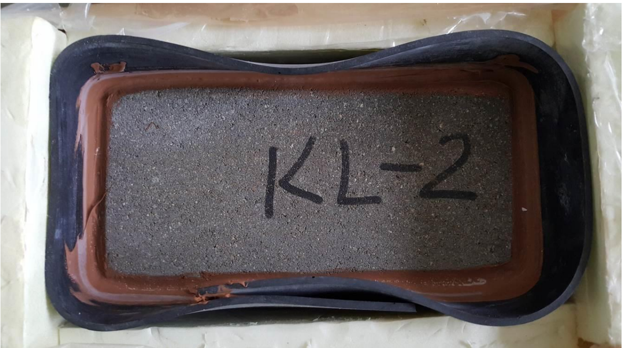
4 Figure Block KL-2 before the freeze/thaw testing (top) and after 72 days of testing (bottom)
